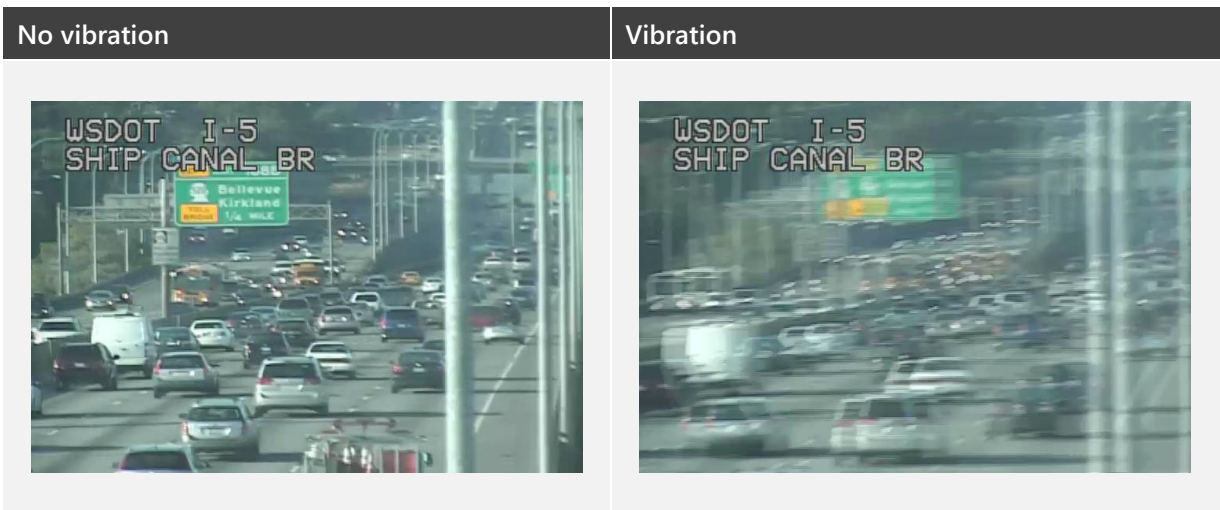
Figure 2-7: Vibration effects on CCTV image
