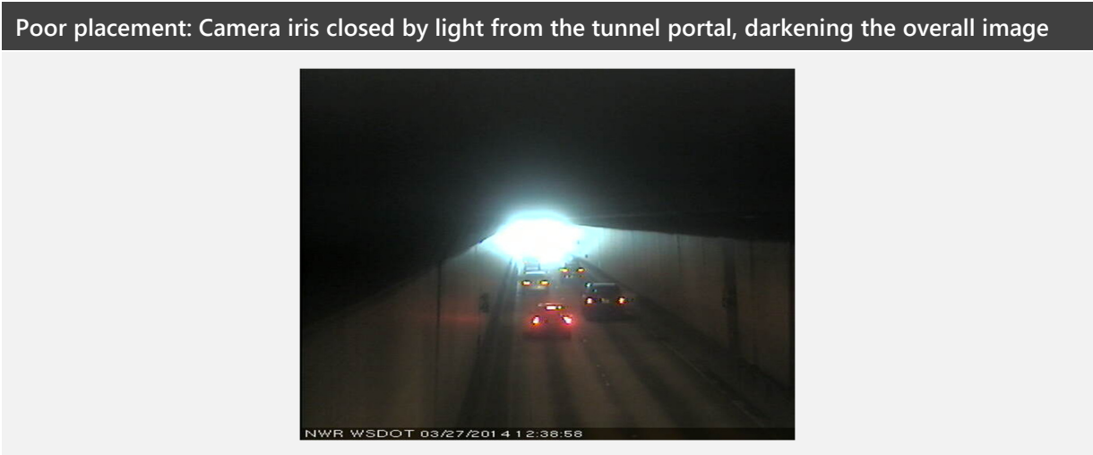
Figure 2-6: Lighting effects on CCTV iris
