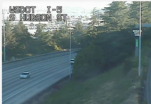
Figure 2-4: Poor coverage due to vegetation growth
